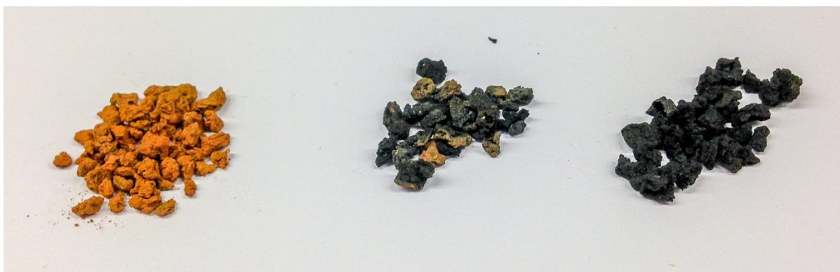
Fig. 5. Different extents of oxidation, ranging from full oxidation (left) to pyrolysis only (right). In the middle sample there is almost no carbon left. The samples correspond to “Sludge Ash”, PA_800_60 and P_550_60 respectively.
