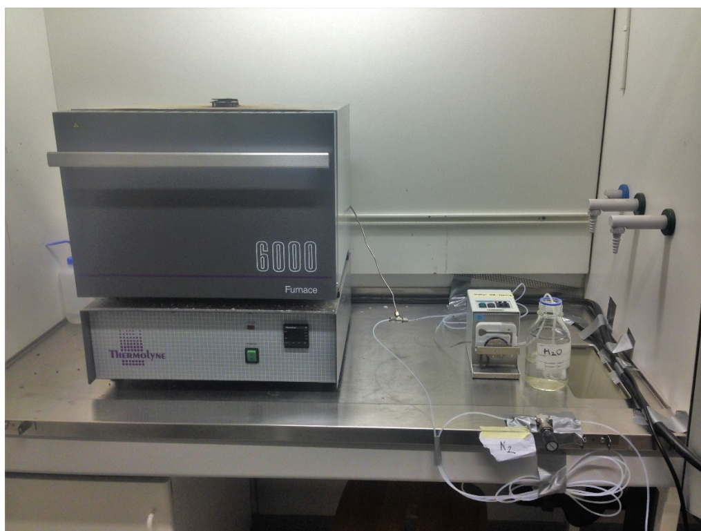
Fig. 3. Experimental set-up. Nitrogen flow control valve is seen in the lower right corner. Above it on the bench is the peristaltic pump. The flows are mixed and enters the back of the furnace through a metal pipe.
