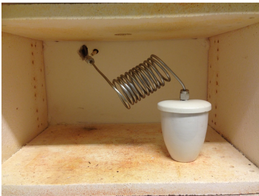
Fig. 4. The inside of the furnace chamber. Nitrogen and water enter the rear of the chamber and is heated in the spiral before entering the crucible through a hole in the lid.
