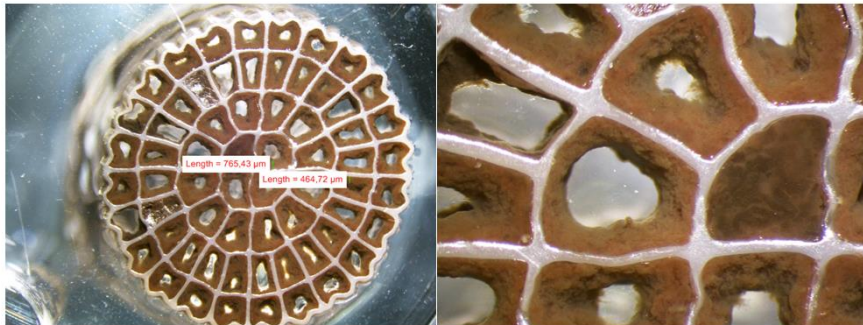
Figure 5. Microscopic photos of a K5 carrier (left) and zoomed-in (right) with a thick biofilm
