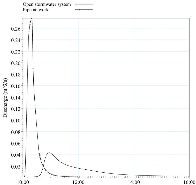
Figure 6-12: Showing the discharge from the open stormwater system and the conventional system at monitoring point 1.
