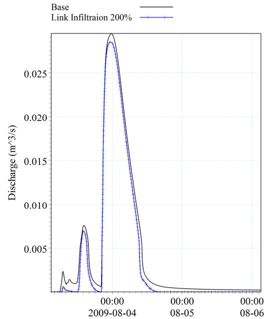
Figure 5-11: Increased infiltration rate in the links results in overall runoff volume.
