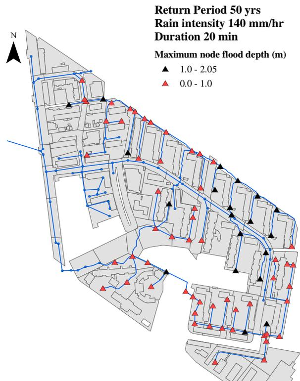
Figure 10: The maximum node flooding in the pipe network system caused by the 140 mm/hr intensity rainfall for the duration of 20 minutes.
