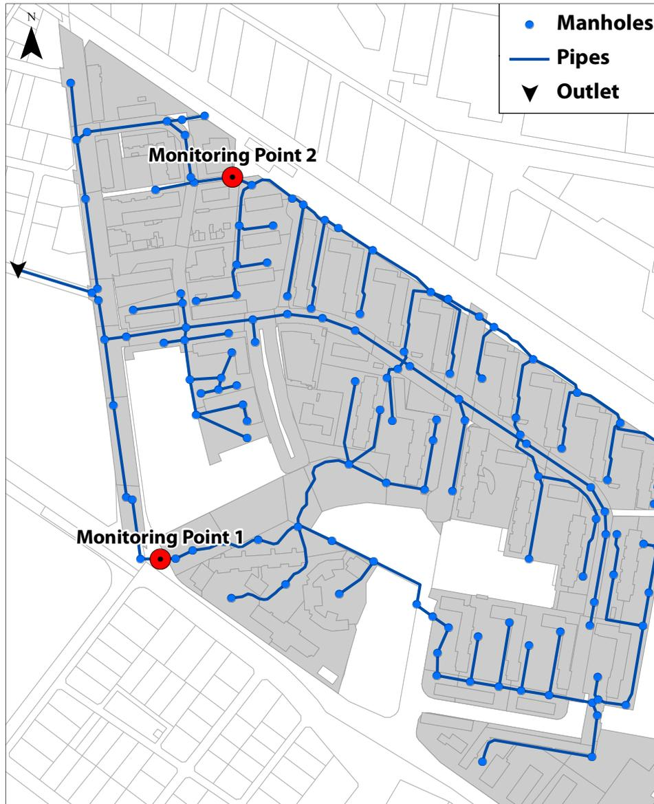
*Figure 6-4: Pipe network model used in Scenario 2 and the location of monitoring points.*
