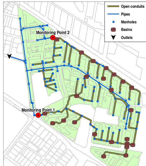
Figure 4: The layout of the hydraulic network of Augustenborg in MIKE URBAN and the location of monitoring points.
