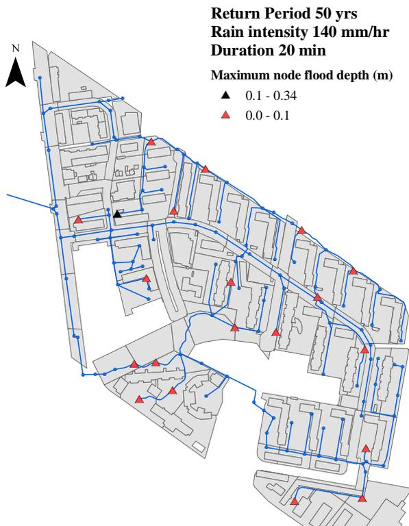
Figure 9: Maximum node flooding in the open stormwater system caused by the 140 mm/hr intensity rainfall for the duration of 20 minutes.
