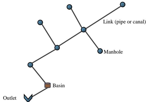
Figure 4-2: Illustrates a basic collection hydraulic network in MOUSE.
