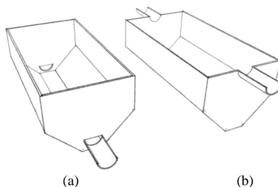
Figure 4-5: An illustration showing a basin with different links configurations to model (a) dry ponds, (b) wet ponds.
