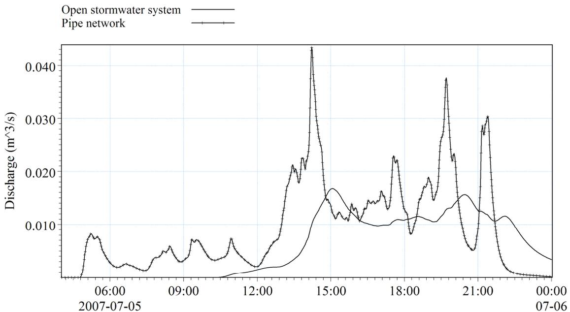
Figure 8: The simulated discharge at monitoring point 1 is plotted for both systems. The open drainage system exhibits a more evened out discharge hydrograph.
