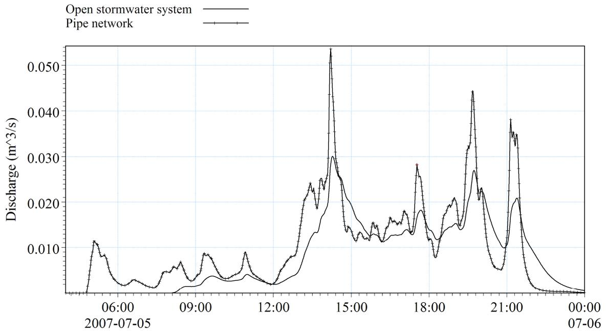
Figure 6-5: The simulated discharge at monitoring point 2 simulated for the open stormwater system compared to the discharge from the pipe network system at the same location.
