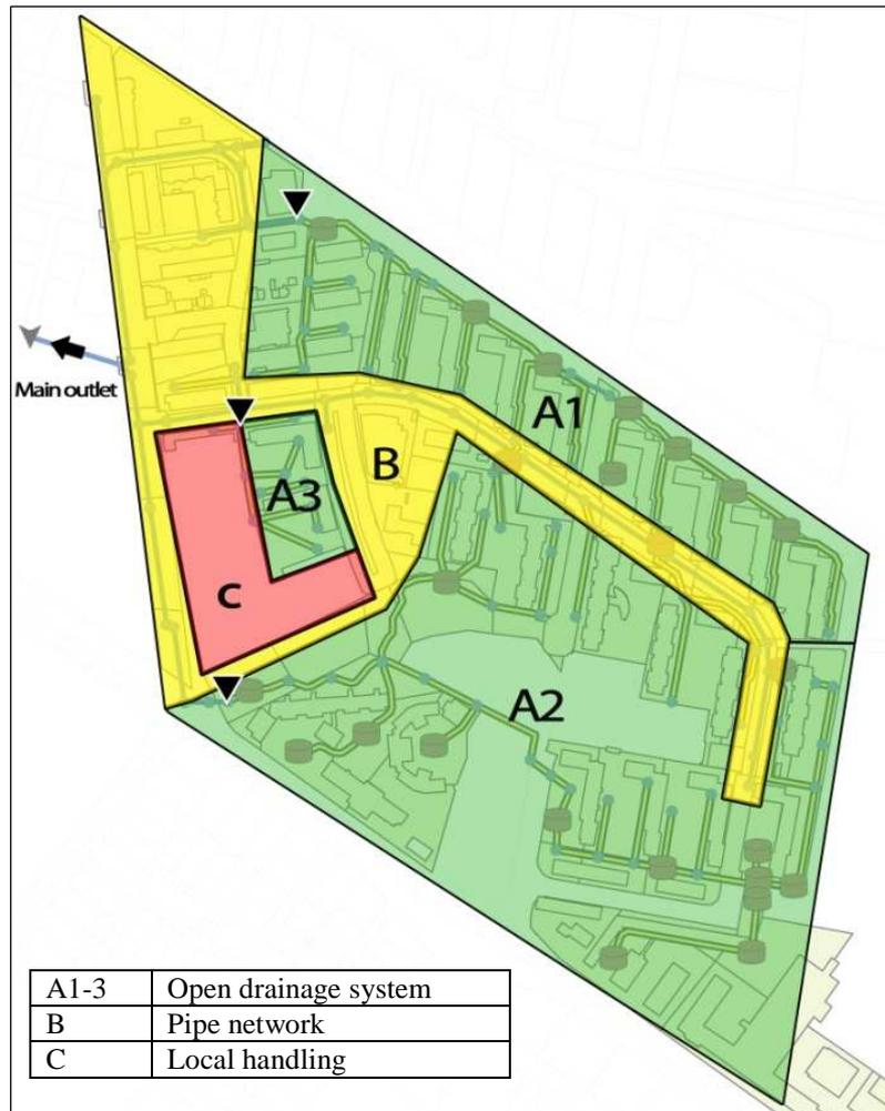
Figure 2-3: Stormwater handling methods in Augustenborg. The triangle symbols show the connection points of the open drainage system to the pipe network.
