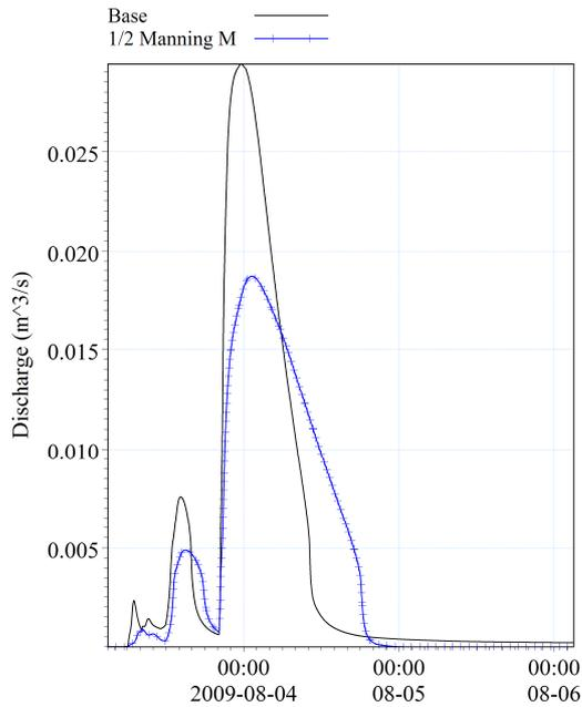
Figure 5-10: Effect of reducing the Manning coefficient to the half for the links in the system.
