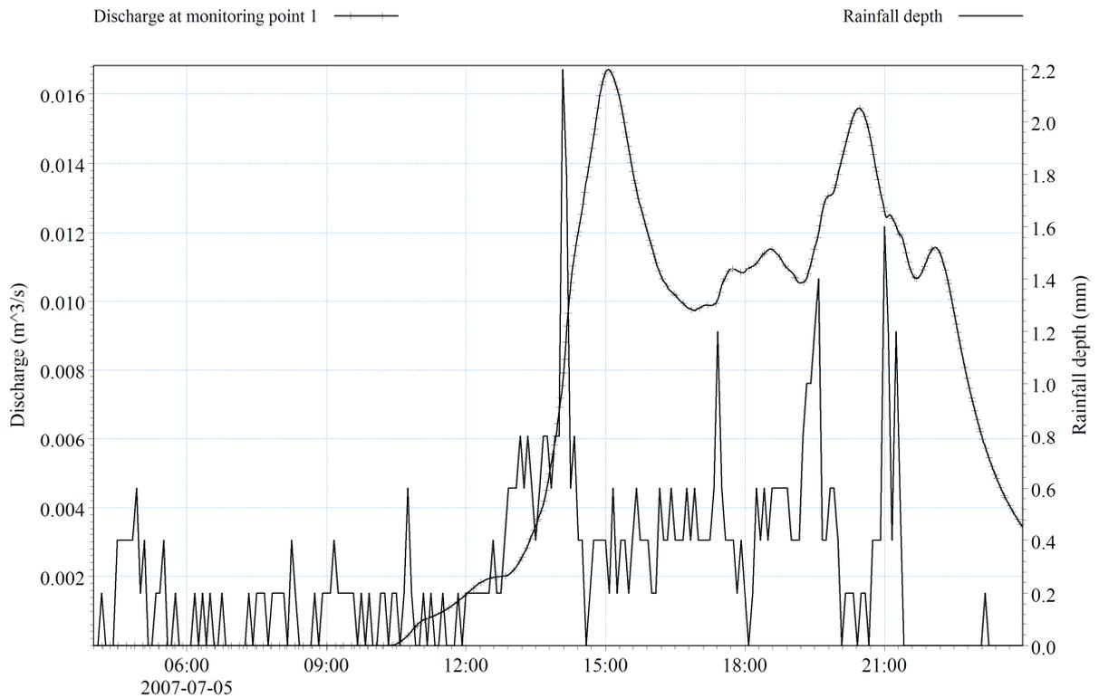
Figure 6-3: The discharge from monitoring point 1 (left axis) plotted against the rainfall depth (right axis, 5 minutes resolution).
