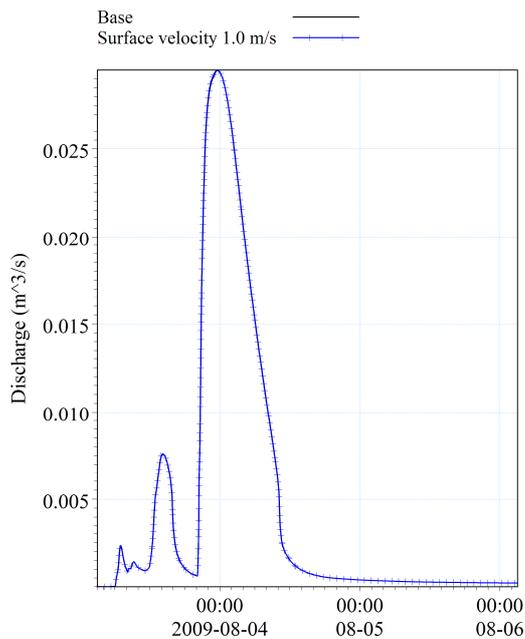
Figure 5-8: No significant change in the discharge hydrograph associated with changing the surface velocity.
