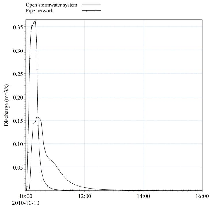
Figure 6-13: The discharge from the open stormwater system compared to the pipe network at monitoring point 2.
