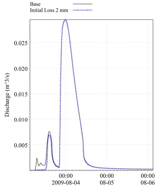
Figure 5-7: Effect of initial loss on the runoff.
