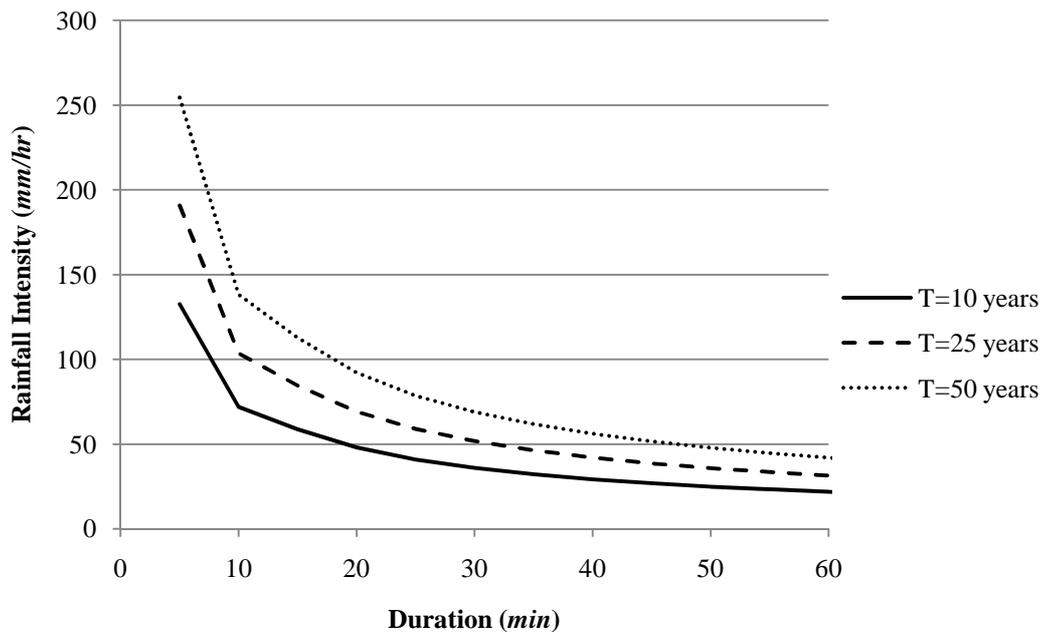
Figure 6-7: Rainfall intensity curves calculated using Dahlström formula for different return periods (T).
