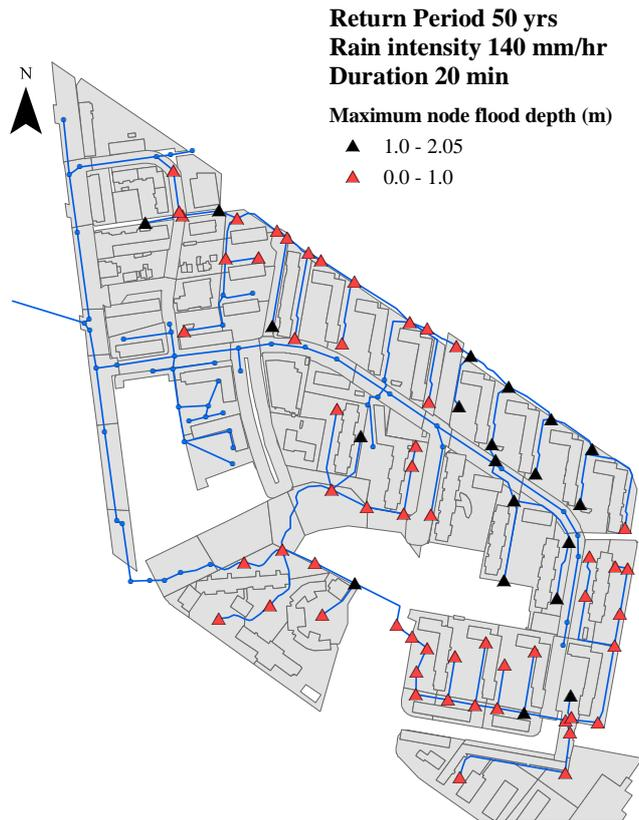
Figure 6-11: The maximum node flooding in the pipe network system caused by the 140 mm/hr intensity rainfall for the duration of 20 minutes.
