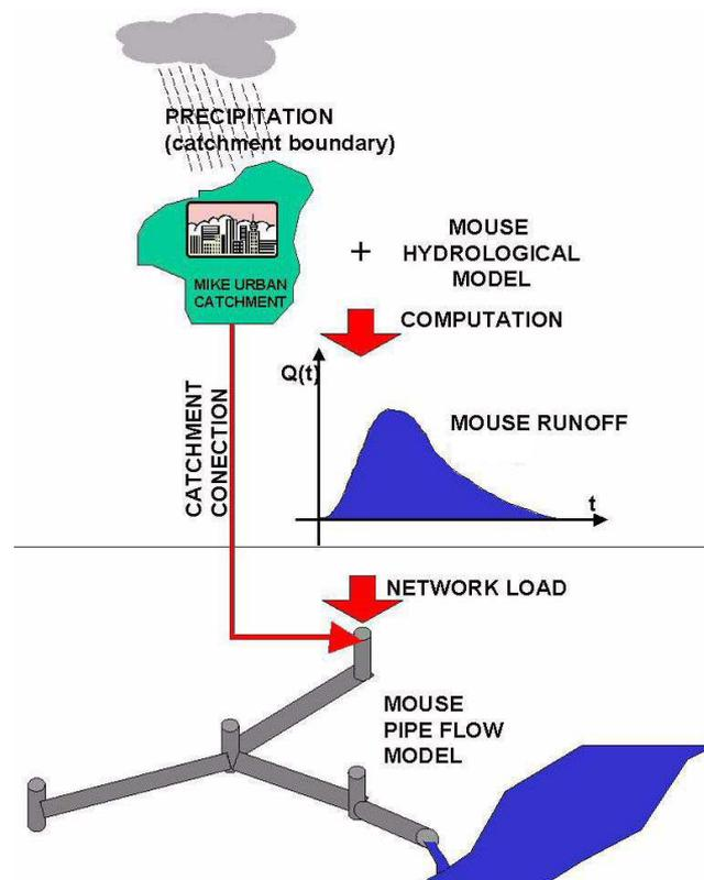
Figure 4-1: Illustrates the concept of modeling a collection system in MOUSE consisting of a hydrological and a hydraulic model (DHI Software, 2009a).
