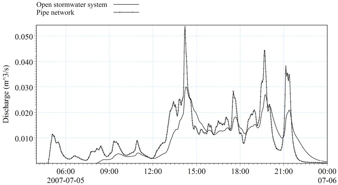
Figure 7: The simulated discharge at monitoring point 2 simulated for the open stormwater system compared to the discharge from the pipe network system at the same location..
