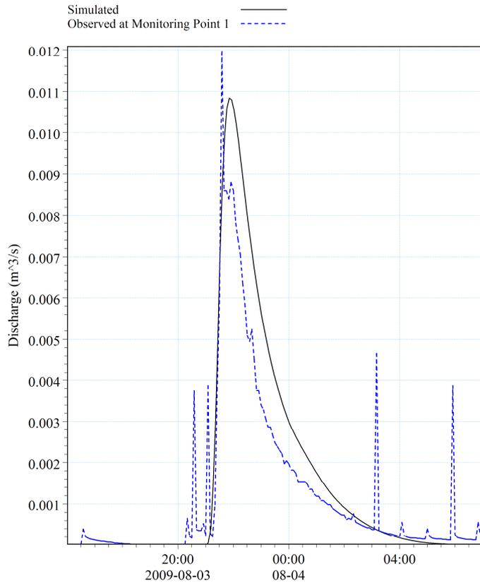
Figure 5-13: The calibration result in monitoring point 1.
