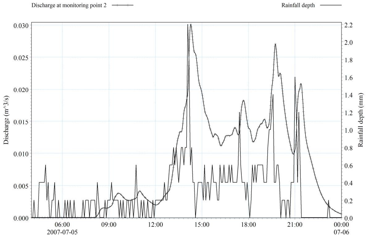
Figure 6-2: The discharge from monitoring point 2 (left axis) plotted against the rainfall depth (right axis, 5 minutes resolution).
