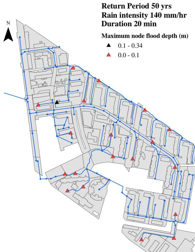
Figure 6-10: Maximum node flooding in the open stormwater system caused by the 140 mm/hr intensity rainfall for the duration of 20 minutes.
