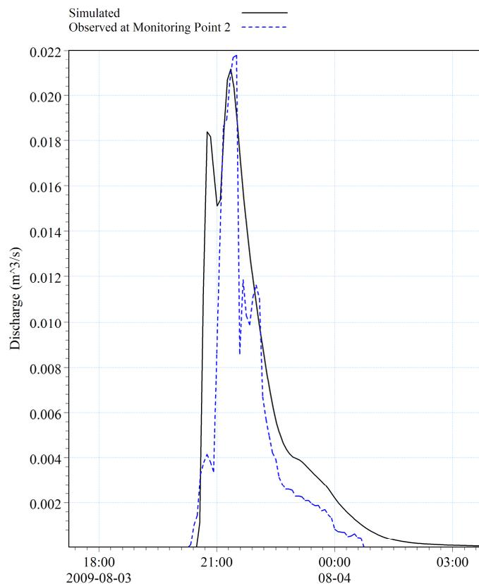
Figure 5-12: The simulated flow at monitoring point 2 compared to the measured flow.
