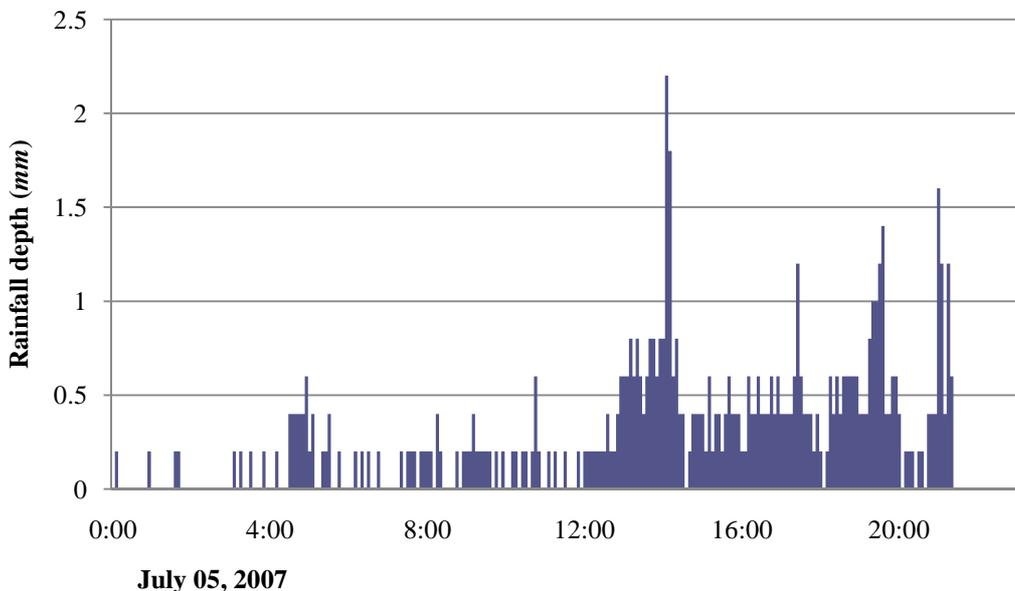
Figure 6-1: The rainfall event used in scenario 1 and 2 (5-min interval).
