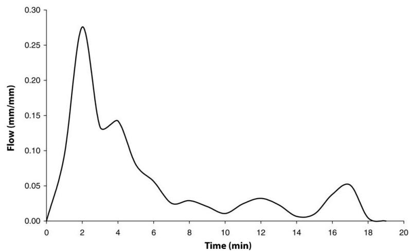
Figure 3-1: Average unit hydrograph (1 mm) (Villarreal & Bengtsson, 2005).
