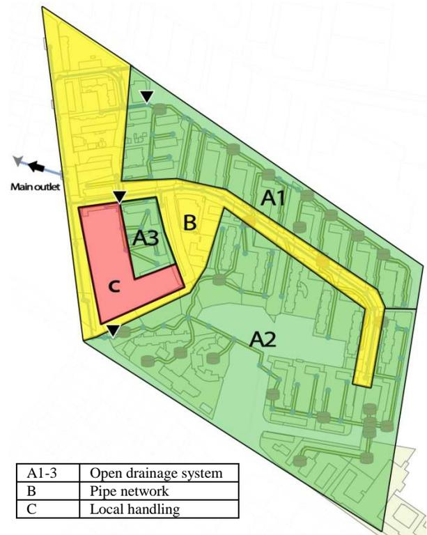
Figure 3: Stormwater handling methods in Augustenborg. The triangle symbols show the connection points of the open drainage system to the stormwater sewers.
