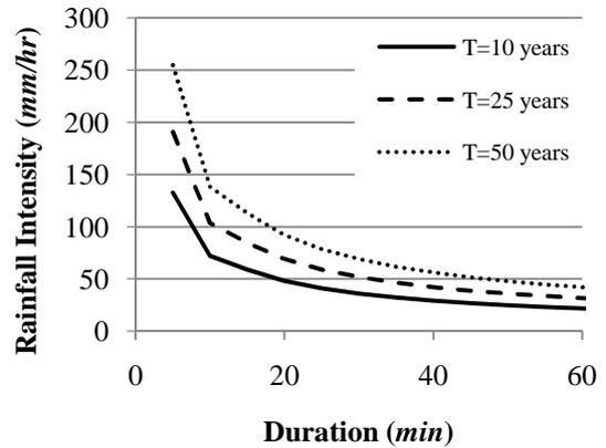
Figure 6: Rainfall intensity curves calculated using Dahlström formula for different return periods ( $T$ ) (Svenskt Vatten, 2004).
