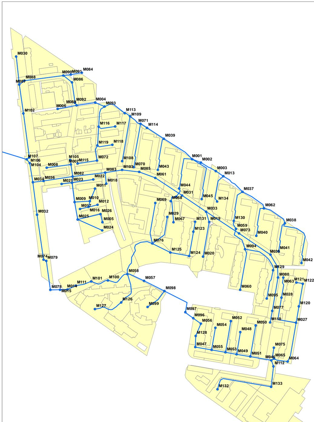
Figure C-2: The pipe network nodes.
