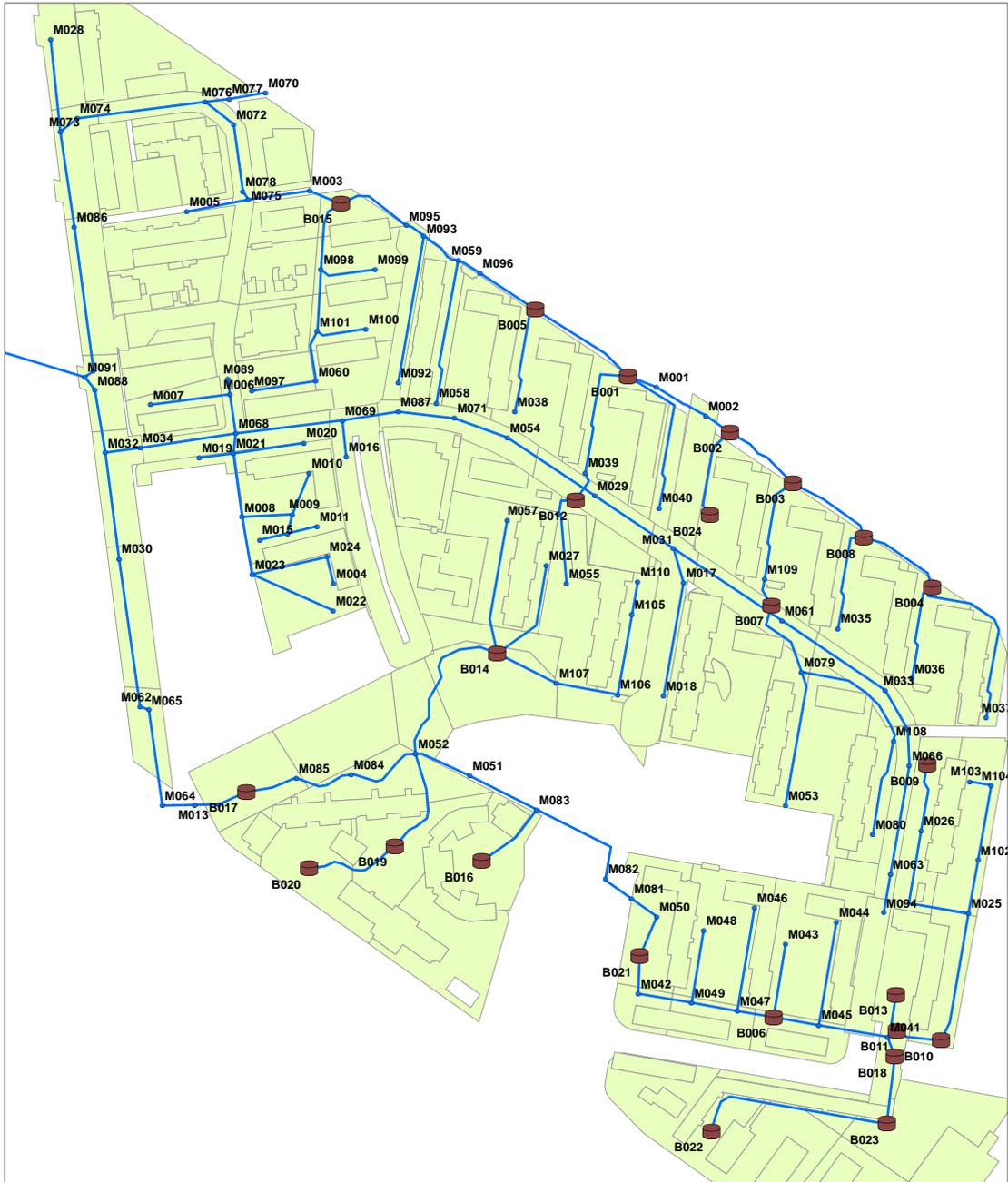
Figure B-2: The nodes in the open stormwater system. “B” indicates a basin and “M” indicates a manhole.
