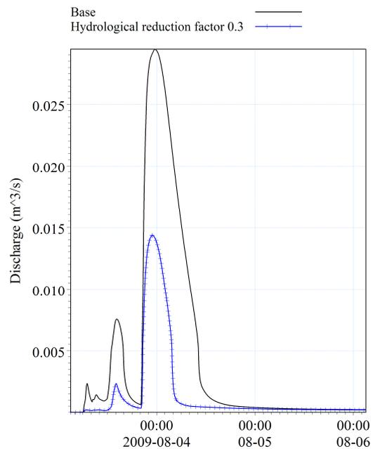
Figure 5-9: The effect of the hydrological reduction factor.
