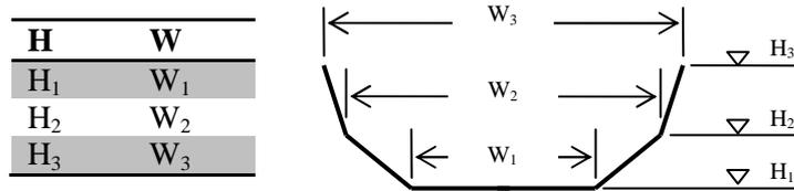
Figure 4-4: Definition of the channel cross-section using the “H, W open” tabulated data.
