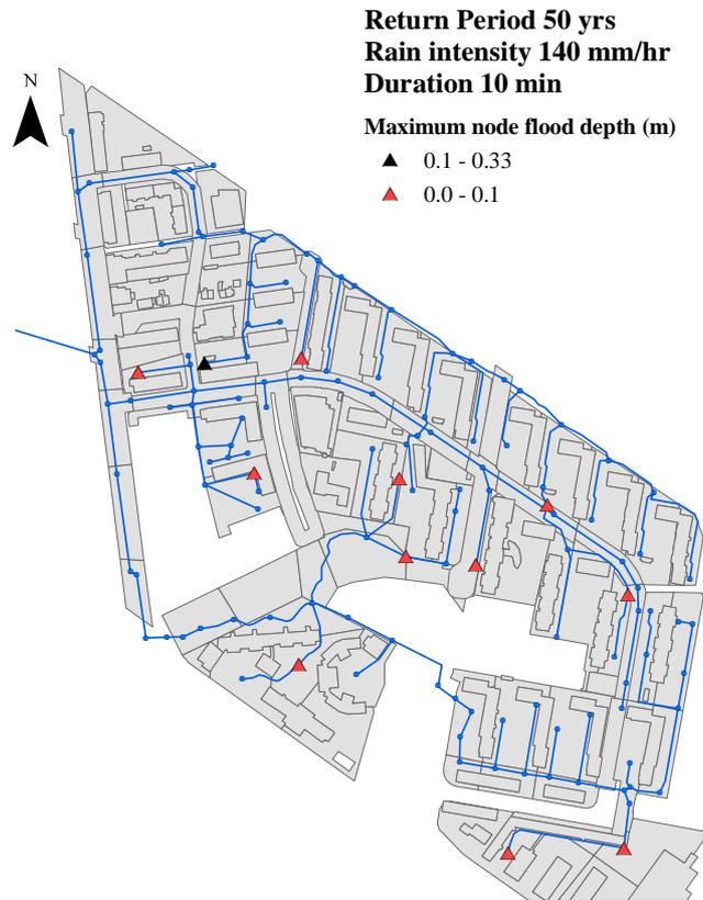
Figure 6-8: The maximum node flooding in the open stormwater system during the simulation period. The flooding depth is calculated as water level – ground level.
