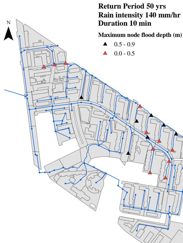
Figure 6-9: The maximum node flooding in the pipe network during the simulation period.
