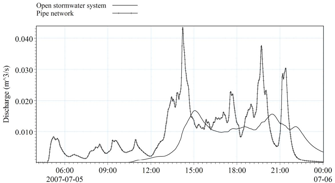
Figure 6-6: The simulated discharge at monitoring point 1 is plotted for both systems. The open drainage system exhibits a more evened out discharge hydrograph.
