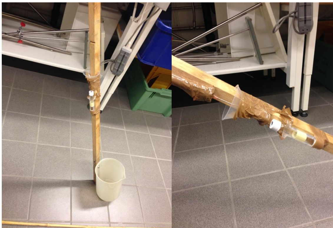
Figure 6: Left. Customized sampling device. Right. Close up on tube holder with the needle stick placed above.
