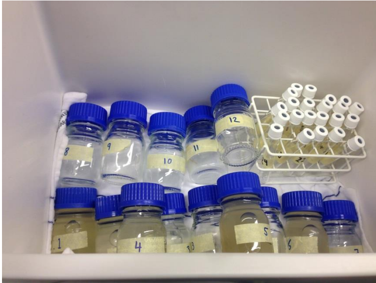
Figure 5: Cooling box filled with ice and a blanket put on top of the ice. 100 ml bottles marked with a number.
