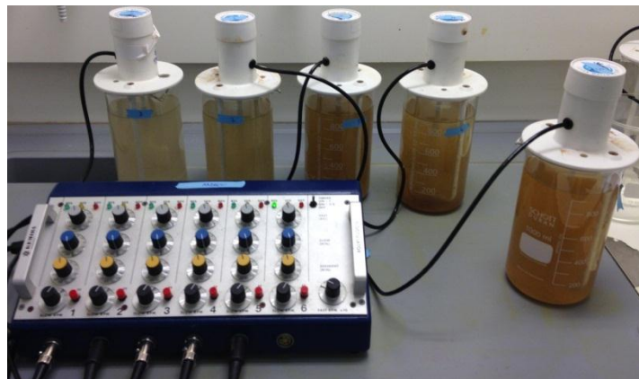
Fig. 3.1 Jar test 1 setup during slow mixing phase
